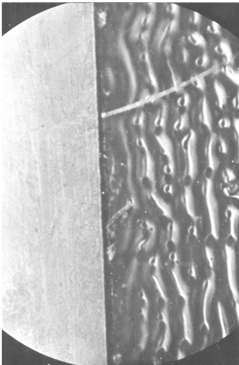
FIGURE 4b The same LC layer subjected to 5 V reveals the existence of a supercritical influence length of a side lateral wall on the secondary electrohydrodynamic instability generated from the flexoelectric one.
