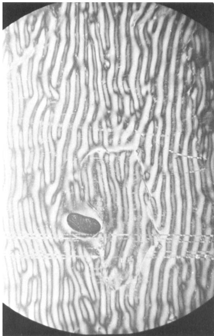
FIGURE 5a Supercritical influence length of air bubbles on flexoelectric surface-induced domains including a hydrodynamic movement of the fluid in a symmetrical weakly-anchored MBBA layer ( 46\ \mu\text{m} ) subjected to 4\ \text{V} ; crossed nicols, the short side of the photo corresponds to 1350\ \mu\text{m} .
